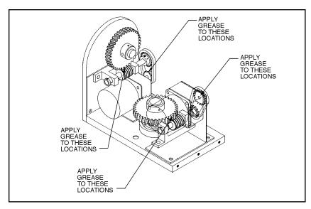
Figure 6. Servicing the Pan/Tilt
